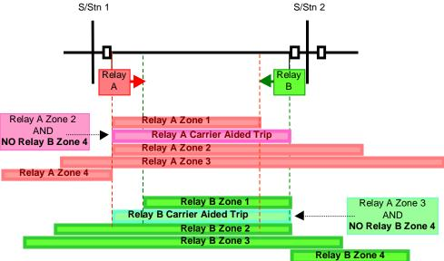
When the Zone 2 instantaneous element picks up, the relay waits for a "blocking signal" to be received. If no blocking signal is received during a set time delay (known as the Permissive Trip Time) the relay will carry out a "Carrier Aided Trip". If, during this time delay, a blocking signal is received, the Zone 2 time delay will remain in place, and the relay will carry out a Zone 2 trip after the Zone 2 Time delay.
