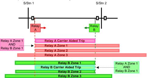
Where the signalling equipment has an output which indicates that the signalling channel is out of service, this can be connected to a Status Input called *Carrier Recv Guard*. On energisation of this status input the relay will revert to a time stepped distance scheme.
