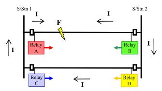
Point F is within the Zone 2 forward reach of relay D, so relay D will send a permissive signal to the remote end, relay C. Relay A will detect the fault in Zone 1, and trip instantaneously.
