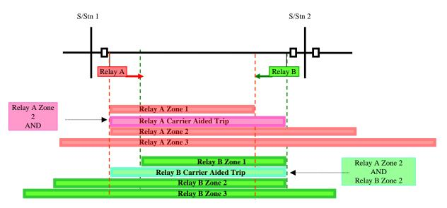
The relay will trip instantaneously for a Zone 1 fault. If a signal is received from the remote end, the time delay will be removed from the Zone 2 element, allowing it to trip instantaneously. The name of the scheme comes from the fact that a <u>Permissive</u> signal is being sent by the <u>Overreaching Zone 2</u>
